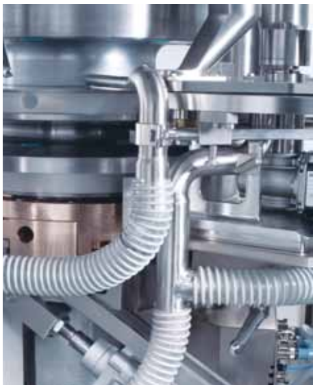
Dust extraction for multi-layer tablets
