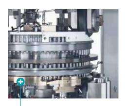
Two identically sized pre-compression and main compression stations on one turret: double capacity
